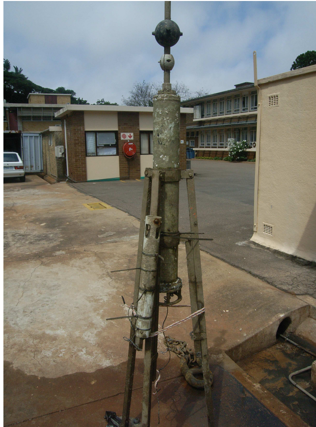
Figure2. Current Meter 1 (Seapac) post recovery.
