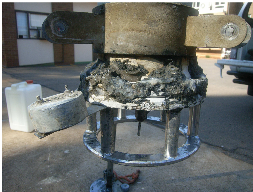
Figure 5. Mud packed around the base on the recovered Seapac (Current Meter1).
