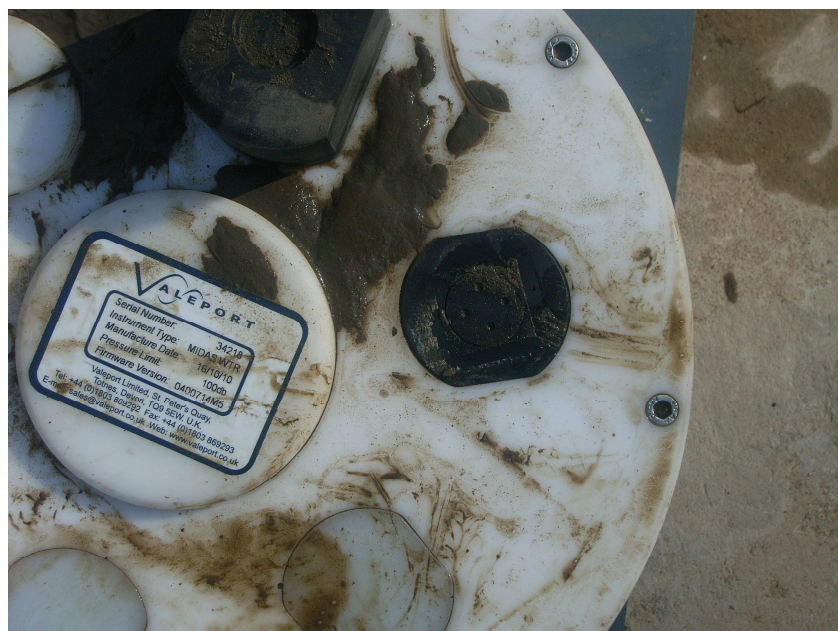
Figure 6. Mud on the top on the recovered Valeport (Wave Meter1).
