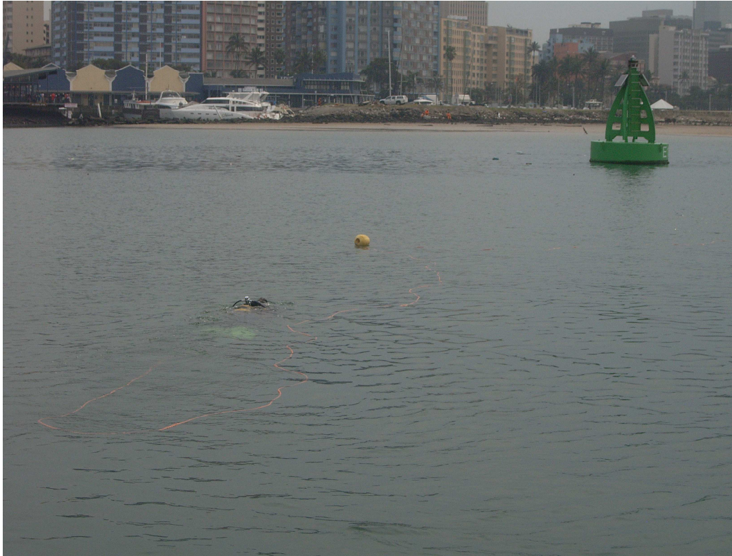
Figure2. Diver preparing to recover WaveMeter 1.
