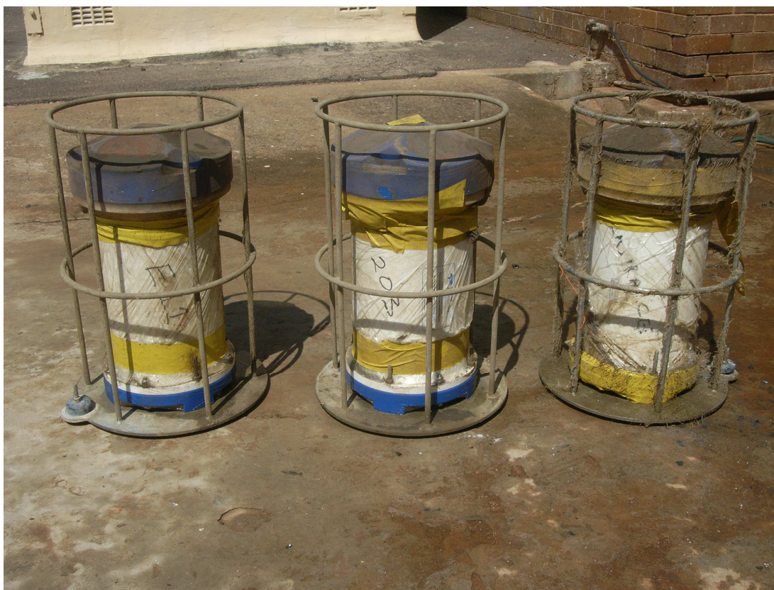
Figure4. The three ADCPs displaying varying degrees of bio-fouling.
